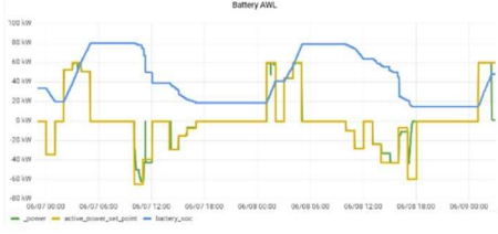
Fig. 5. Results of the optimization algorithm for flexibility provision by the BES connected to node O7:27.
